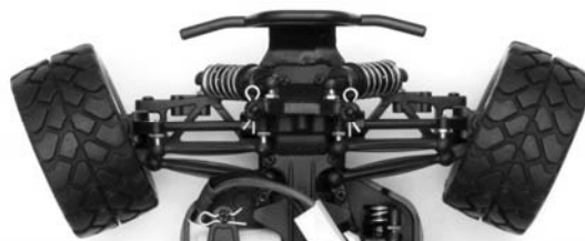
Exaggerated Toe-Out Setting (never run this much!)
