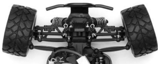
Exaggerated Toe-In Setting (never run this much!)
