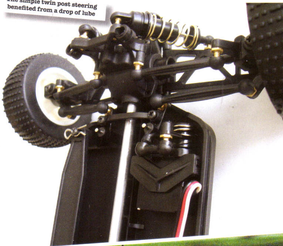
With all the weight down low grip roll is minimised
